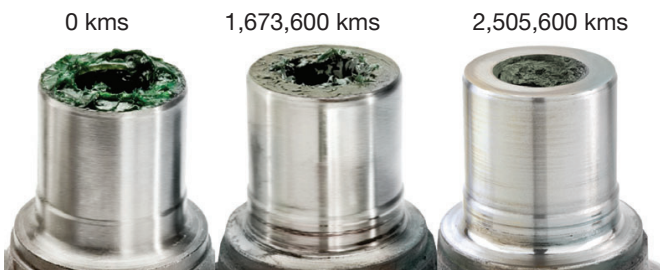
Real life examples of high kilometer U-joints show virtually no wear.
